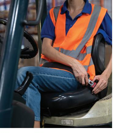
IF YOUR EQUIPMENT IS OUTFITTED WITH RESTRAINT DEVICES, SUCH AS SEAT BELTS, OPERATORS ARE REQUIRED TO WEAR THEM.
